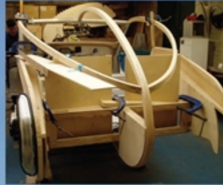
ABOVE: The laminated roof trusses of the prototype AeroMax.
