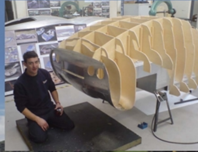
LEFT: The 'egg box' construction which shows the panel maker the exact shape of a prototype body, in this case the LIFEcar.
